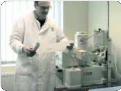
The 'industry standard' equipment for measuring extensibility is the Extensograph.
